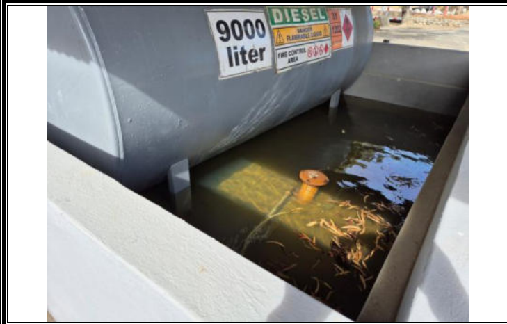
Integrity test of the diesel depot bund
